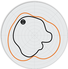
Figure 2. R350 2.4GHz Azimuth Antenna Patterns
