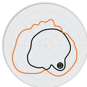
Figure 3. R350 5GHz Azimuth Antenna Patterns
